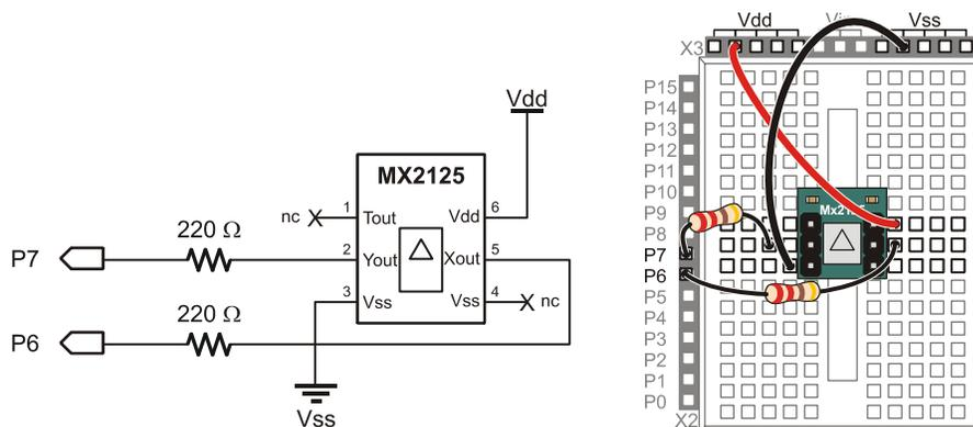
The program below, SimpleTilt.bs2, simply measures the pulse width, that is, the duration of  $t_{Hx}$ , for each axis. The raw values are displayed in the BASIC Stamp Editor's Debug Terminal. If you run the program, then tilt the accelerometer, you should see the values for each axis change.
