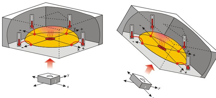
By tilting the accelerometer, the hot gas will collect closer to some of temperature sensors. By comparing the sensor temperatures, both static acceleration (gravity and tilt) and dynamic acceleration (like taking a ride in a car) can be detected. The MX2125 converts the temperature measurements into signals (pulse durations) that are easy for microcontrollers to measure and decipher.
